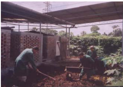
Box Type Composting (Source: Waste Concern)
